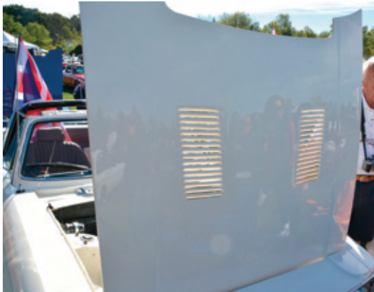
Additional cooling is achieved with louvres in the bonnet - Image: Terence McKillen
