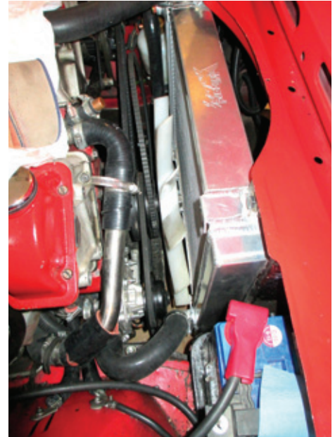
New silicon lower hose connecting pump to new radiator. The power steering pump is removed for clarity - Image: Tanya Duke
