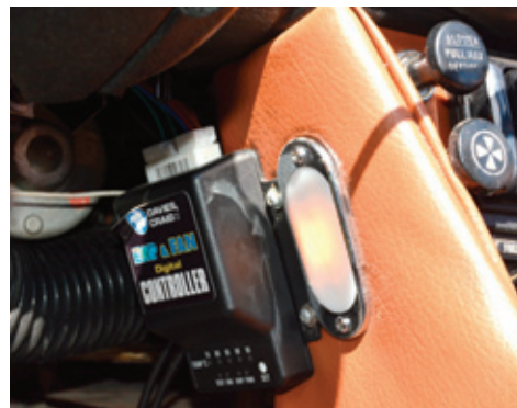
Chris located the pump & fan controller on the side of the centre console - Image: Terence McKillen
