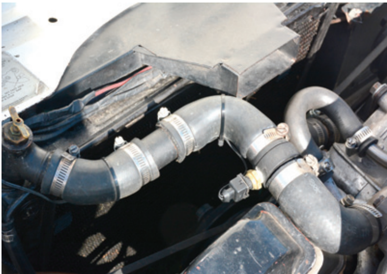
The Davies Craig system is controlled by a digital probe in the upper hose - Image: Terence McKillen
